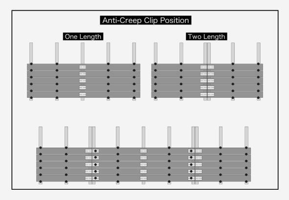
Leave the penultimate row open and move on to the last row of slats, installing them using the same method as the first row. Position the staves, slide the expansion clips into the grooves and slide them to the correct position, then screw them to the slats.
