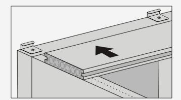
Then, after positioning the first row, place the clips at the top of each stave (clips per stave), these will separate the first row from the second row by determining the lateral distance.
