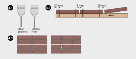
Boards must be fixed with screws in correspondence with each joist. Every board end must be fixed with two screws. If necessary, double the joist.
