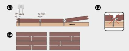
Boards must be fixed with screws in correspondence with each joist. Every board end must be fixed with two screws. If necessary, double the joist.
