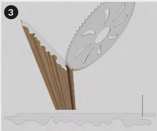
Cut the new panel as shown in the figure, removing the lip of the "female" joint.
