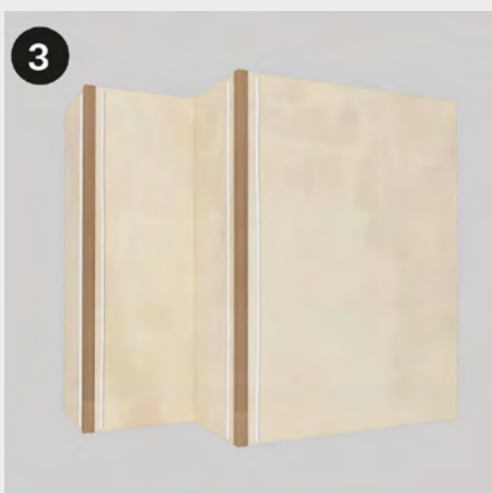
3 Keep applying wall adhesive starting from the outer corners of the wall.
