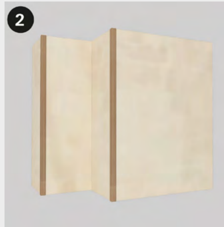
2 Glue the first corner on the outer corners, pressing lightly to secure them in place.
