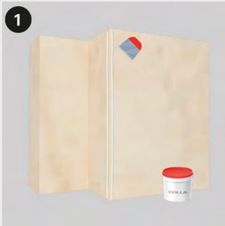
1 Apply wall adhesive starting from the outer corners of the wall.
