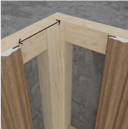
Image 5 shows the inner corner in detail. Measure the remaining space between the last panel and the inner corner: cut the panel according to the measurement obtained considering the size of the male and female joints.
