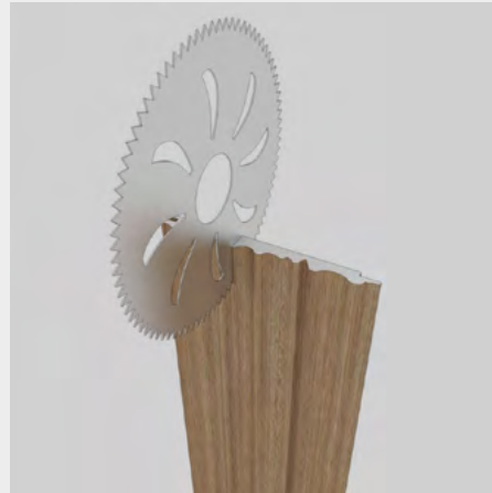
Image 5 shows the inner corner in detail. Measure the remaining space between the last panel and the inner corner: cut the panel according to the measurement obtained considering the size of the male and female joints.
