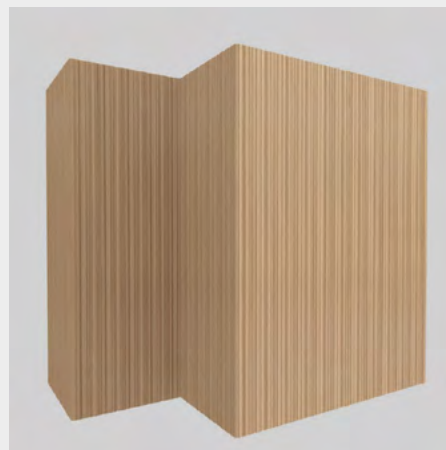
On the other side, measure the distance between the inner corner and the last panel and cut the panel according to the obtained measurement. Place the cut panel after applying the specific glue on the horizontal joints.
