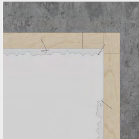
Install the cut panel by attaching it to the joints with the appropriate brads at a 45-degree angle.
