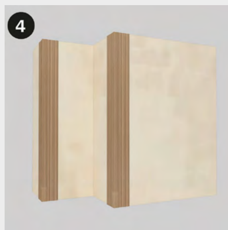
4 Glue the first module adjacent to the newly installed corner profile, pressing lightly to secure it in place.
