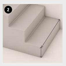
Measure the height and length of the first rise of the step to be covered. Cut a plank of Clap! to size to cover the rise.
