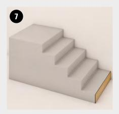
Spread a generous amount of glue on the back of the staves, proceed first with gluing the vertical riser.
