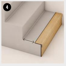
Lay the previously trimmed staves to the step and measure the uncovered part of the tread.
