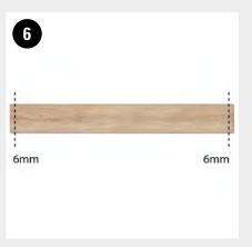
When cutting, always ensure that you leave at least 6mm per side along the length of the staves. For example: stair width 1m--> stave width 0.988 m
