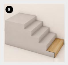
Complete the step by fitting and gluing the tread trim.
