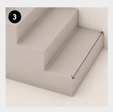
Measure the width of the stairway and cut the Clap!Step profile to length according to the measurement obtained.
