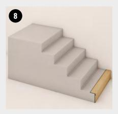
Proceed, taking care to always leave 6 mm of air along the edges of the step, then glue the Calp!Step product and complete the step by fitting and gluing the tread trim.
