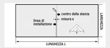
Drawing the installation line. Start from the center of the room. Parallel offset the line using the X measurement as distance.
