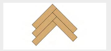
Install the strips precisely and in the order indicated by the numbers on the strips. Carefully check the joints between the strips after every strip that is added. Note! No protruding edge may be felt!
