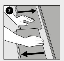
Disassemble the individual slats by sliding them along the short side.
