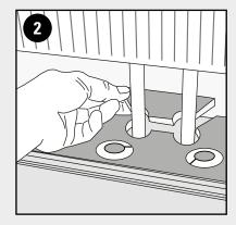
Drill holes at least 15 mm wide in relation to the diameter of the pipes. Remove a small section of stave in order to position the stave. Cover the remaining space behind the pipes with the section removed earlier.
