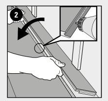
Place spacers between the last plank and the wall.
