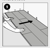
Push the installed planks towards the front wall on which the 15mm spacers were previously positioned.
