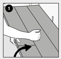
Lift the entire row by carefully tilting it upwards. Slide up the long side.
