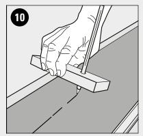
Place a spacer and measure the width of the surface to be covered. Cut the slats to size making sure you never have slats less than 50mm wide.
